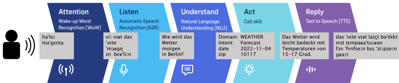
Figure 1: The main flow of a digital voice assistant: detect the Wake-Up-Word, transcribe speech to text, classify text as intents and recognize entities, execute some service, and generate speech output as a response.
